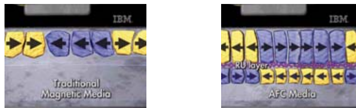
Fig. 5. Schematic representation of AFC media with single magnetic transition.
