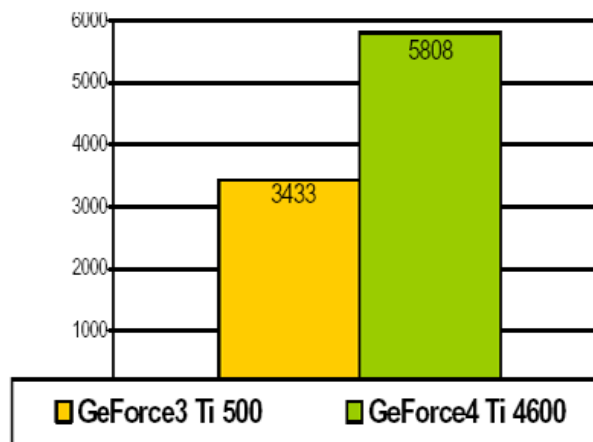
This chart shows comparison of performances of GeForce4 Ti 4600 and its predecessor in FPS.
