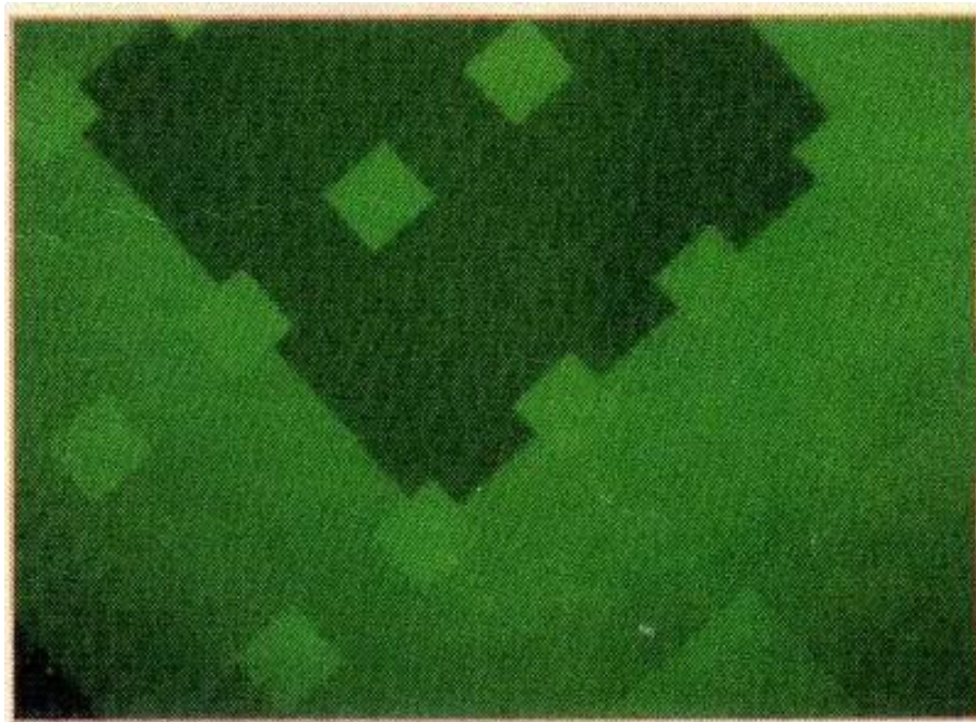
Figure 4. A Fluorescence microscope image of a patterned 1,500 \mu m x 1,500 \mu m protein-resistant plasma polymerized tetraglyme (pp4G) pad on a silicon-dioxide substrate, with additional 200 micron x 200 micron gold pads on and around the PP4G pad, after incubation in a solution containing fluorescently labeled proteins.
